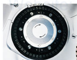
Reaction Tray 37±0.1°C, real-time monitor.
