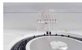
Washing Probe Independent 7-step washing system.
