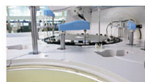
Mixer Probe Dual mixer, auto frequency adjustment
