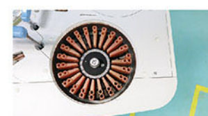
Reagent Tray 2~8°C cooling for 24 hours
