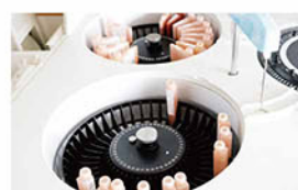
Reagent Tray 2~8°C cooling for 24 hours.
