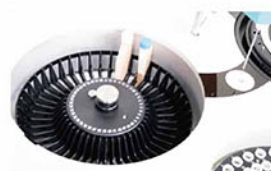
Reagent Tray 2~8°C cooling for 24 hours.
