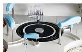
Reaction Tray 37±0.1°C, real-time monitor.
