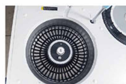
Reaction Tray 37±0.1°C, real-time monitor.
