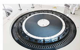
Reaction Tray 37±0.1°C, real-time monitor.
