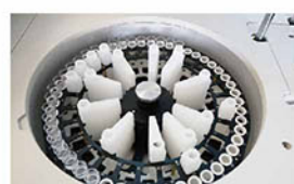
Reagent Tray 2~8°C cooling for 24 hours.
