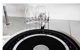
Washing Probe Independent 7-step washing system.
