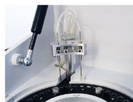
Washing Probe Independent 2-step washing system.
